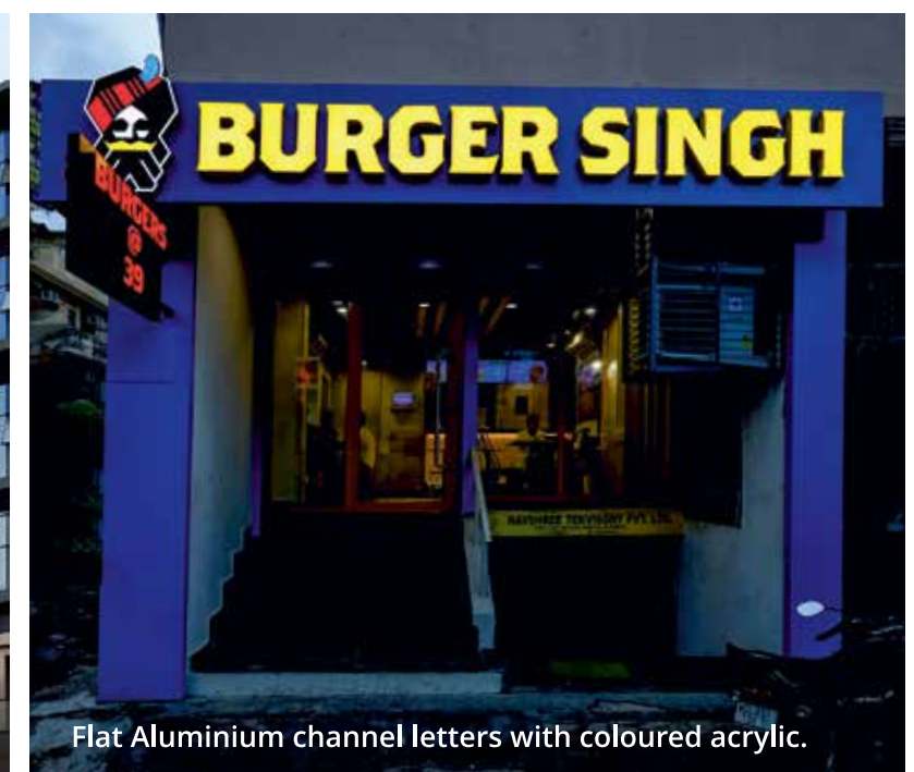
3M vinyl pasted on side aluminium channel letters as per the design.
